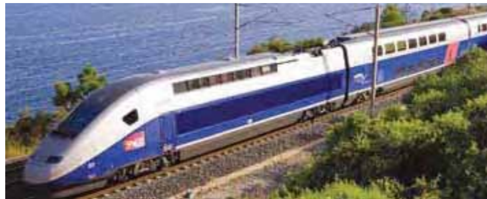
Figure 1 The French TGV (Train à grande vitesse) electric train can reach speeds of more than 500 km/hour
