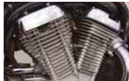
Figure 2 Motorcycle engine fins
