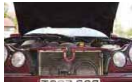
Figure 1 A car radiator helps to transfer energy from the engine
